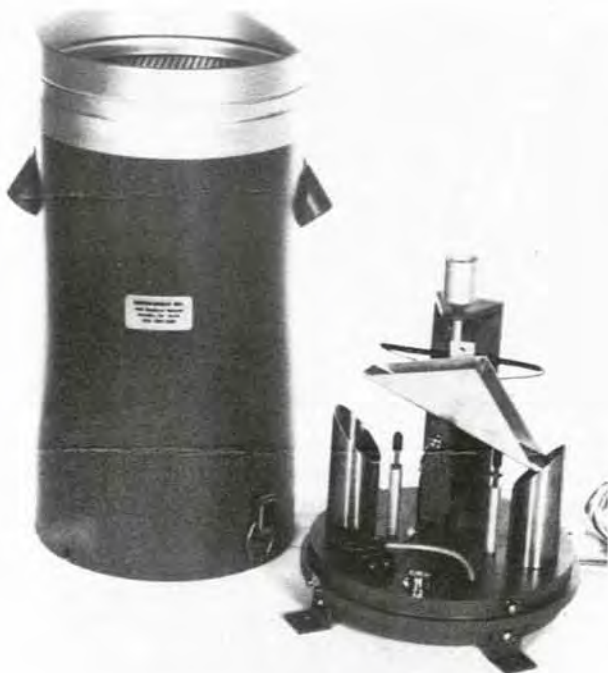
Figure 9.10—Self-draining tipping bucket rain gauge; model with 8-inch-diameter orifice. (Photo courtesy of Sierra-Misco, Inc.)
