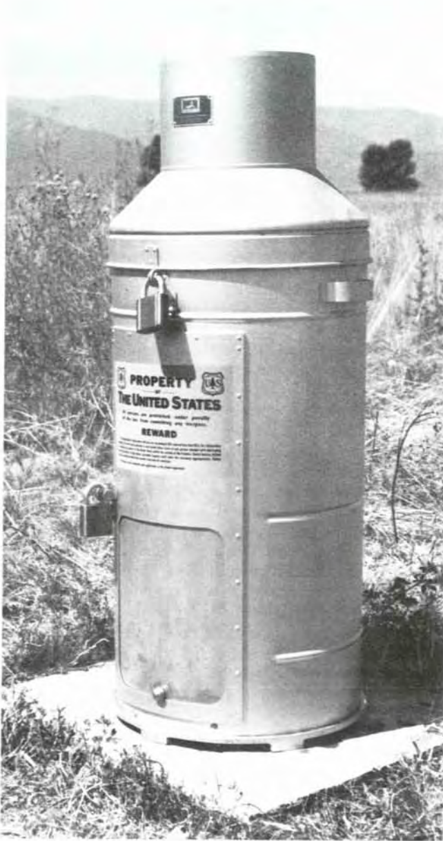
Figure 9.6—Universal weighing-type precipitation gauge: left, assembled gauge; right, weighing and recording mechanisms.
