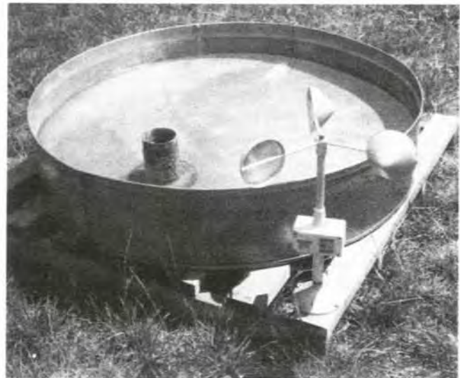
Figure 12.1—Class A evaporation pan on wooden support, with installed accessory equipment: stilling well (containing fixed-point gauge), submerged-mount Six's thermometer, and totalizing anemometer. (Photo from National Weather Service.)
