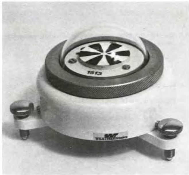
Figure 11.2 —Black and white pyranometers: Eppley model (top, photo courtesy of Sierra-Misco, Inc.); star pyranometer (bottom, photo courtesy of Qualimetrics, Inc.).
