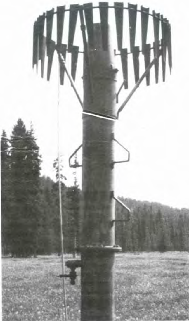
Figure 9.15—Standpipe storage precipitation gauge, with Alter shield. (Photo from National Weather Service.)
