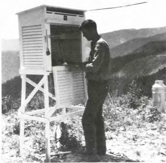
Figure 7.1—Cotton region instrument shelter; the standard design in use at manual fire-weather, climatological, and evaporation stations.
