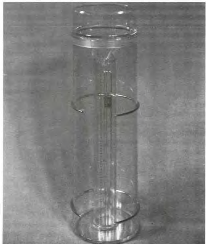
Figure 9.5 —Four-inch clear plastic direct-reading rain gauge.
