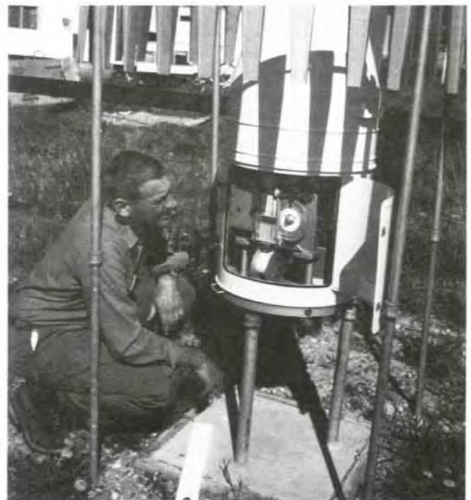
Figure 9.8 —Punched-tape recording precipitation gauge, a digitally recording type of weighing gauge.
