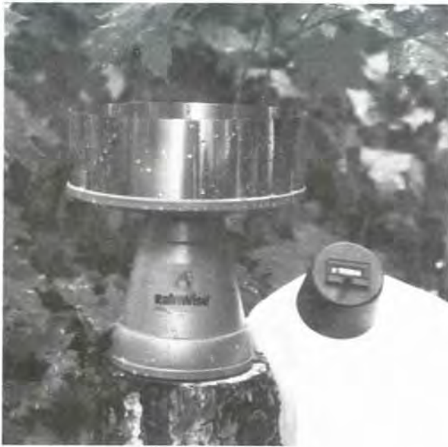
Figure 9.12 —Electronic rain gauge, self-draining tipping-bucket type, with digital counter. (Photo courtesy of RainWise Inc.)
