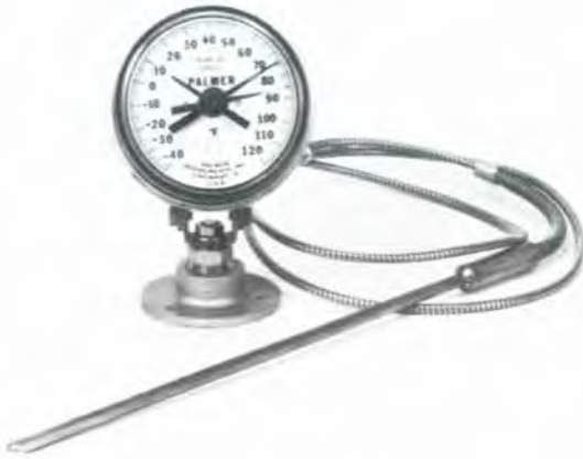
Figure 13.1 —Soil maximum-minimum thermometer, similar to thermometer in figure 7.10 but with 5-ft flexible armor capillary tubing connected to mercury-in-steel sensing probe. (Photo courtesy of Palmer Instruments, Inc.)
