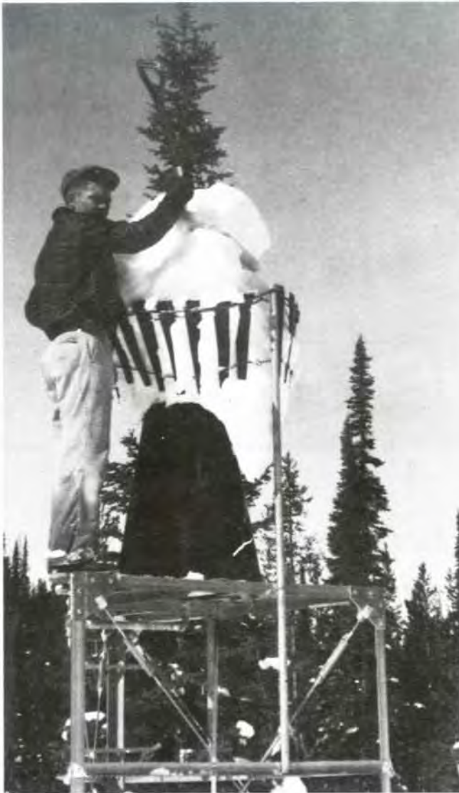
Figure 9.17 —Snow buildup that may occur between Alter shield and sloping wall of Sacramento storage gauge, particularly with shield of previously used configuration (see text). (Photo from National Weather Service.)
