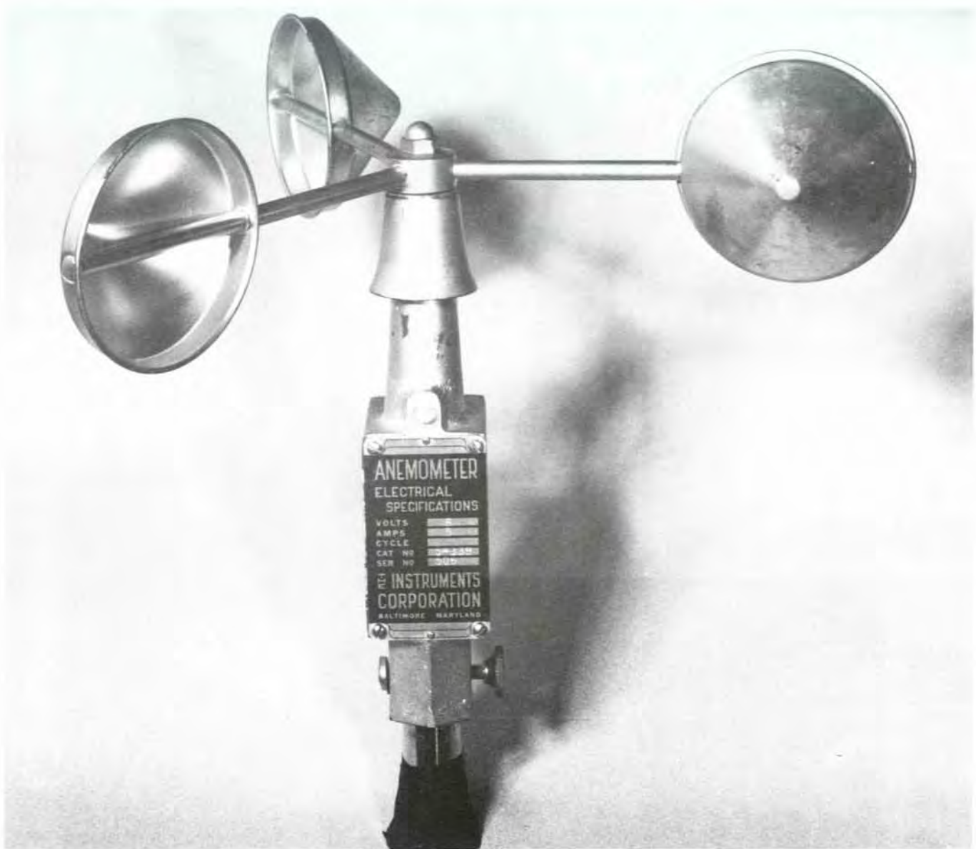
Figure 8.2—Small Airways anemometer with \frac{1}{60} -mile contacts, used at many fire-weather stations.
