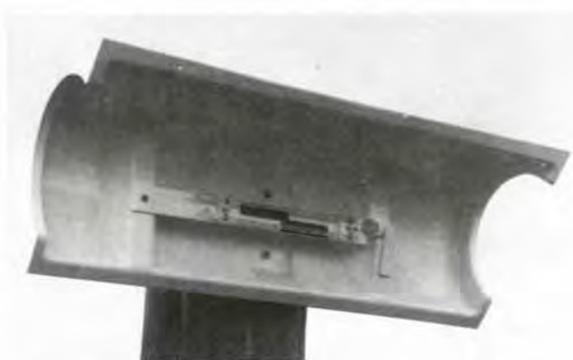
Figure 7.6—Orchard type shelter, made of molded plastic. (With mounted Six's type maximum-minimum thermometer.)
