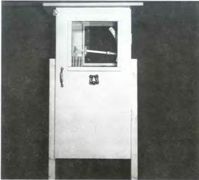
Figure 10.2 —Forester (Appalachian) fuel moisture scale mounted in Appalachian scale shelter.
