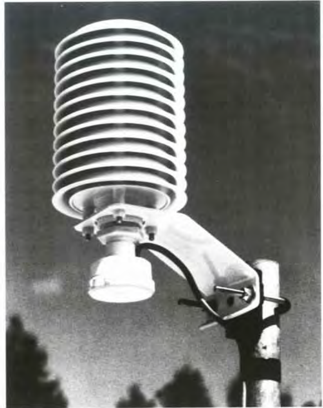
Figure 7.2—Gill multiplate solar radiation shield (R.M. Young Company); naturally ventilated type made of plastic, used with electrical or electronic temperature and humidity sensors. (Photo courtesy of Sierra-Misco, Inc.)
