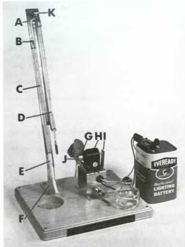
Figure 30.6 —Standard electric fan psychrometer, Forester Model 9X060 (left) and Forest Service model (right): A, thermometer mounting frame; B, thermometer retaining clip and screws; C, wet-bulb thermometer; D, dry-bulb thermometer; E, wet-bulb wick; F, support bracket; G, fan and shaft; H, motor; I, thrust plate; J, fan bushing; K, spacer screw.
