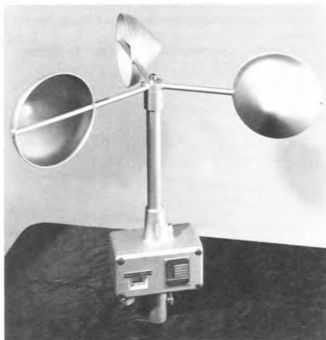
Figure 31.7 —Belfort totalizing anemometer: A, cap nut; B, hub screw; C, cups; D, housing; E, back cover plate; F, spindle retaining screw; G, spindle; H, upper ball bearing; I, worm gear; J, worm wheel with pins; K, terminal block assembly; L, thumbscrew.
