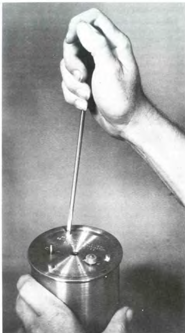
Figure 30.14— To correct for backlash and drag between gears, loosen three screws on bottom of drum and shift gear away from center of drum.
