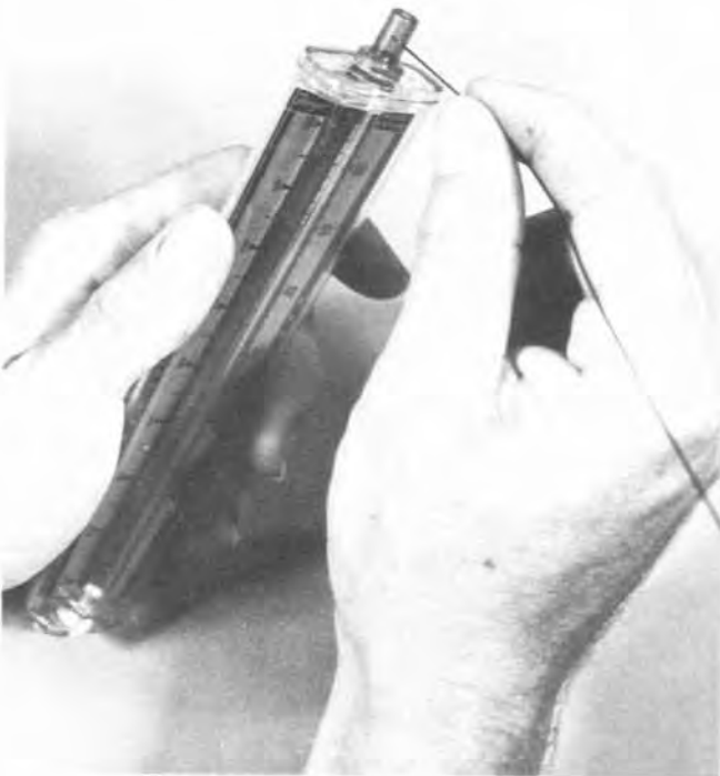
Figure 31.11—Top: cleaning, drying, and removing static from inner tube of Dwyer meter. Bottom: cleaning top stem pinhole.
